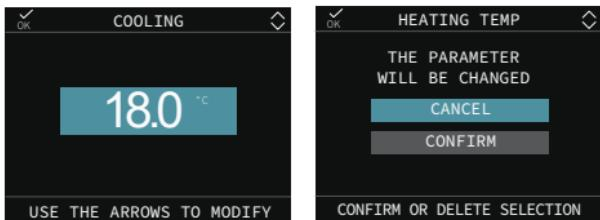
When cooling temperature adjustment is activated, the delivery temperature value is automatically selected by the system, which quickly adjusts the ambient temperature according to the variations in the outdoor temperature. If you want to change the temperature value from that automatically calculated by the electronic board, the COOLING setpoint can be modified within the range (-5 to +5) to obtain the required comfort level.
