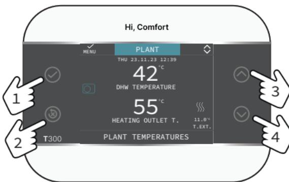
The four side keys described below allow you to easily carry out all the operations necessary for programming and customizing the device.
