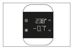
To access the offset modify screen, hold down the way key in the main screen until the blinking °C symbol appears, then press the key again. The correction value is displayed on the large digits and can be changed with the // keys; the small digits show the measured temperature to which the selected correction is applied. The new value must be confirmed by pressing the button. Alternatively, if you press , the current value is restored.
