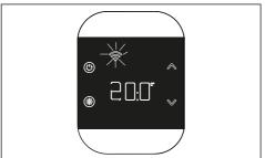
If the symbol "" is off, this indicates that the procedure has failed and un-pairing must therefore be repeated.
