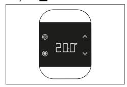
To pair the T200 device with a system, the pairing mode must be activated on the T300 (refer to the RF parameter described into T300 instruction manual for the PAIRING procedure), and then press the key inside the lower casing.
