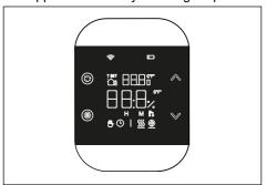
Once the symbol test is complete, the firmware version of the T200 appears on the display for a few seconds. The first line identifies the revision of the RF module (e.g. 6.0), while the second line identifies the FW Host of the object (e.g. S01).
