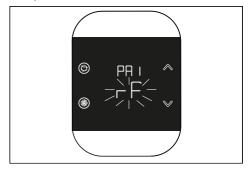
If the procedure is successful, the message OK appears on the T300 while the display automatically switches to the operating screen on the T200 and the symbol "remains on; if the procedure is not correctly completed, the message KO appears on the T300 and the display on the T200 shows the message RTF (Reset To Factory) with the corresponding RF display indicating that pairing was not successful.
