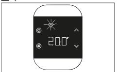
Otherwise, if the T200 is paired with a T300, but communication is not yet present (waiting for first message or loss of connection), the symbol "" is off.
