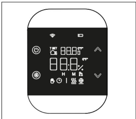
Once the symbol test is complete, the firmware version of the T200 appears on the display for a few seconds. The first line identifies the revision of the RF module (e.g: 6.0), while the second line identifies the FW Host of the object (e.g: S01).
