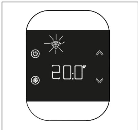
If the symbol “” is off, this indicates that the procedure has failed and un-pairing must therefore be repeated.
