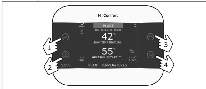
The four side keys described below allow you to easily carry out all the operations necessary for programming and customizing the device.
