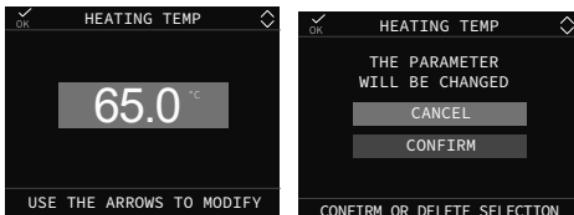
When an outdoor temperature sensor is installed, the outlet temperature is automatically selected by the system, which quickly adjusts the ambient temperature according to the variations in the outdoor temperature. If you want to change the temperature, raising it or lowering it with respect to that automatically calculated by the electronic board, it is possible to change the HEATING setpoint selecting the desired comfort level within the range (-5 to +5).
