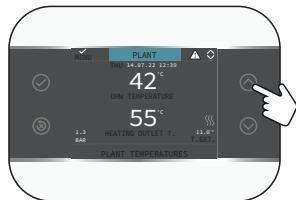
Press the button until the symbol is highlighted to access the anomaly description screen.
