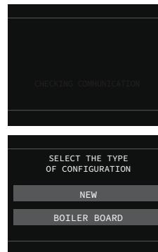
If the communication test is successful, the T300-Hy prepares for the system type configuration.
