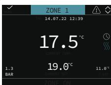
It is also possible to set the T300-Hy as a room controller. In this mode, if POR = 1, in addition to setting the start and end times for each time slot (up to a maximum of 4 slots per day), it is also possible to configure a room temperature setpoint (SETP).
