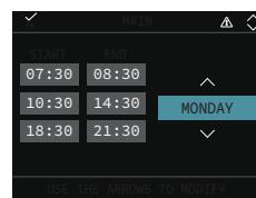
Two time programmes are available with the heat pump: one for Winter and one for Summer. Select the desired season (HOT WATER ONLY or HEATING AND HOT WATER) from MENU/STATE/SYSTEM.
