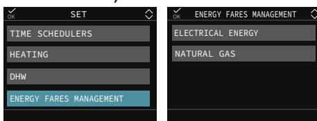
To maximize system efficiency, it is possible to customize the energy cost based on your supply contract. You can assign up to 3 price bands for each type of supply (3 for electricity – 3 for natural gas).
