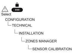
set the desired ambient temperature correction offset.
